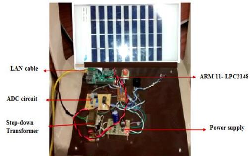
Fig. 13. Prototype of Embedded Industrial System
