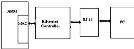
Fig. 10. ARM interfaced with Ethernet Controller
