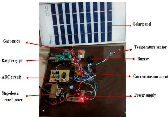
Fig. 2. Prototype of Embedded Controller Unit
