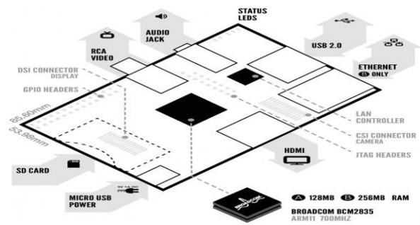
Fig. 9. Raspberry Pi Architecture
