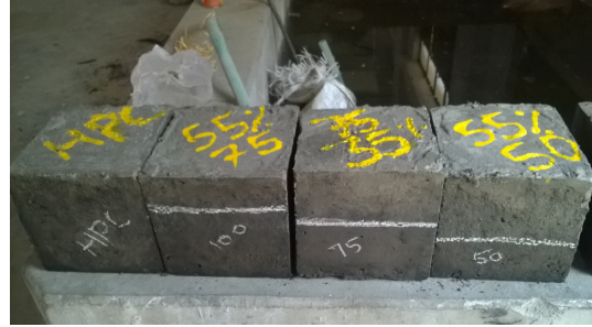
Figure 2 Concrete cubes with varying interface
