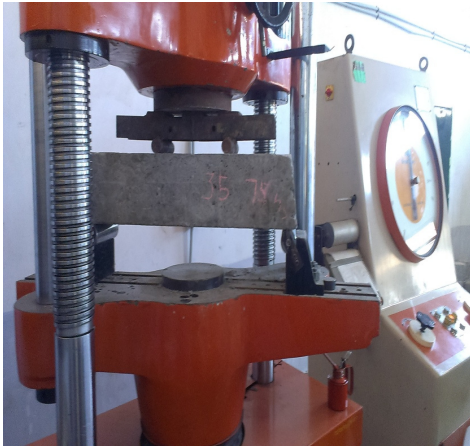
Figure 9 Testing of flexural strength of prism
