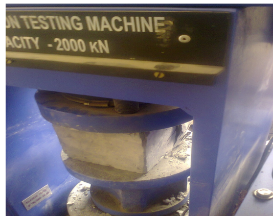
Figure 8 Testing of cubes (2000kN capacity)
